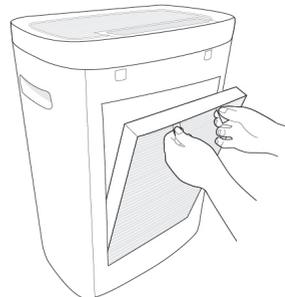
3. To insert the filter into the purifier, put the filter into the main casing with the side that has the handles facing outwards.
