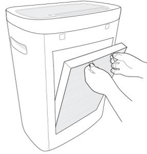
4. Hold the back cover of the purifier; insert the bottom hooks of the back cover into the bottom slots of the purifier; and then push the back cover against the purifier to reattach the back cover firmly.
