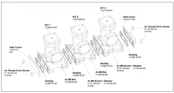
Figure 4: Example assembly for one system with three modules (kits)
