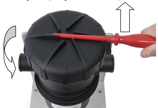
Fig. 17 Opening lid of ProVent 400 (2)
