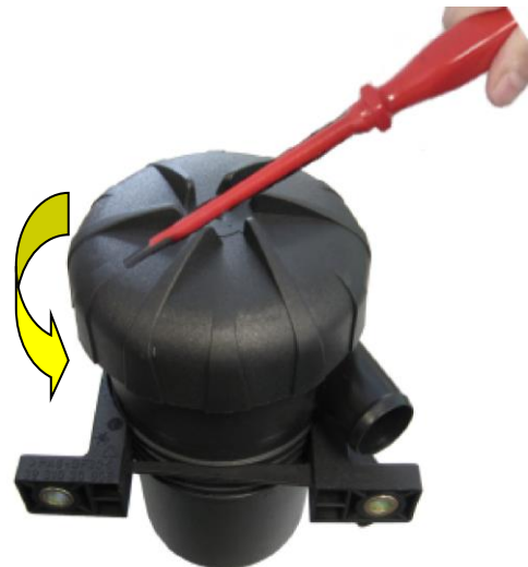
Fig. 14 Detaching lid of ProVent 200
