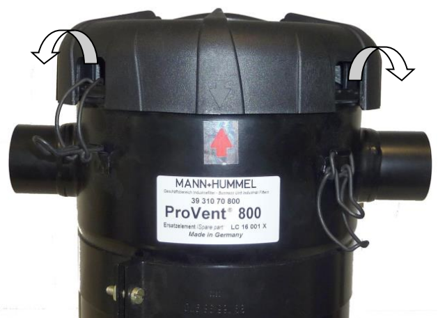
Fig. 21 Opening quick-connect couplings of ProVent 800
