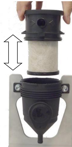
Fig. 13 Changing oil separator of ProVent 150
