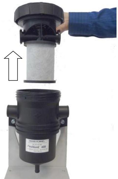
Fig. 18 Removing oil separator of ProVent 400
