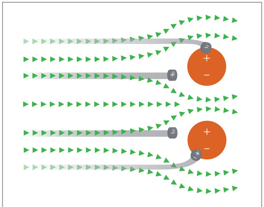
As the dust builds around the media fiber the electrostatic charge is masked. But as mechanical filtration (in this case straining) is increased, there is no significant loss in overall efficiency.
