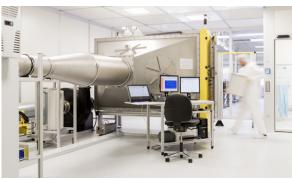
▲ EN 1822 test facilities are essential to ensure the quality and performance of HEPA filters
