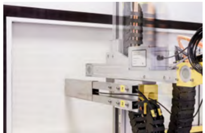
HEPA filter panel during the scan test
