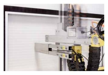
HEPA filter panel during the scan test
