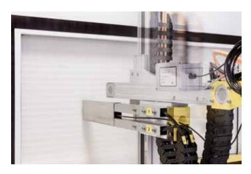
HEPA filter panel during the scan test
