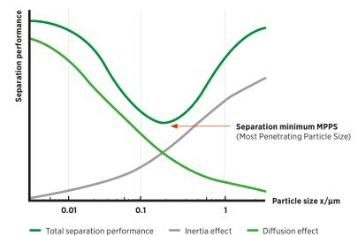
EN 1822:2019 This European filter test standard is our basis for testing and classifying HEPA filters.
