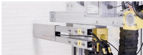
HEPA filter element during the scan test
