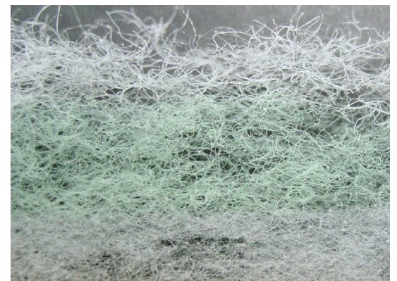
Cross section of Tri-Dek's progressive density media. Air flow travels from top to bottom.
