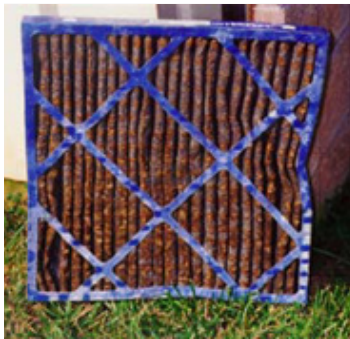
Example of moisture damage and microbial growth
