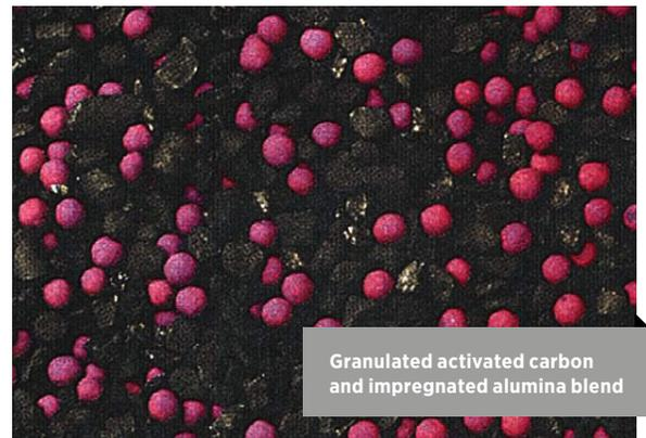
Granulated activated carbon and impregnated alumina blend
