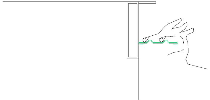
Fig. 14: Bag cords on sealing lip-profile, sealing lip in green
